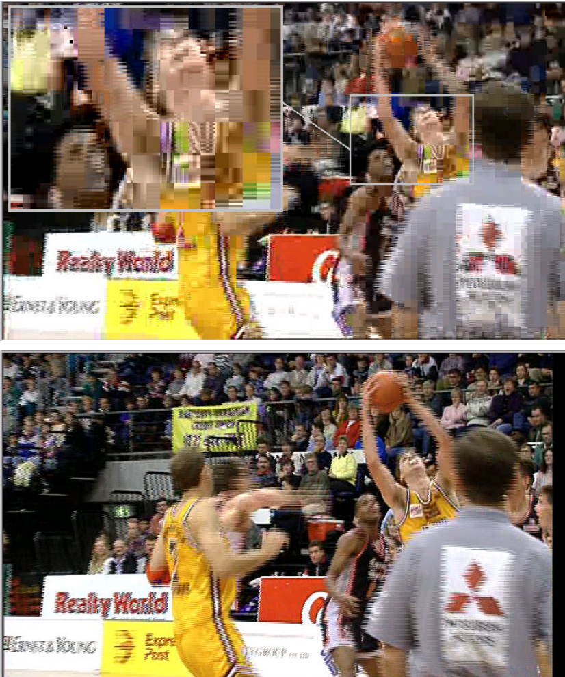
FIG 5: Clearly visible blocking effects on digitally coded TV picture and – by comparison – picture without blocking
